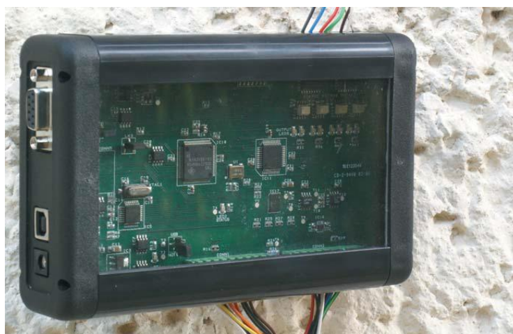
Figure 4.17 TCIC DAQ Board: TCIC Interface Card with on-board electronic cold junction [49].
